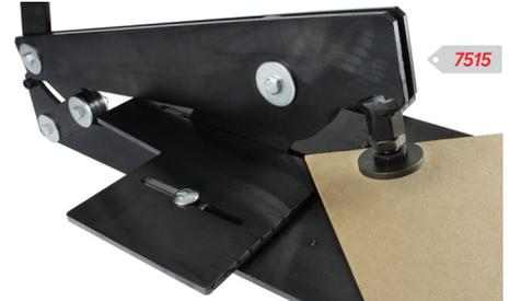
Place backing board in PG-28. Adjust back gauge to give suitable position for pressure pad
