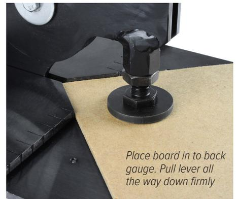
Place board in to back gauge. Pull lever all the way down firmly
