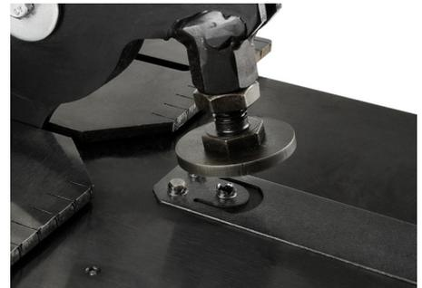
Position strut, spikes up, on spring pegs
